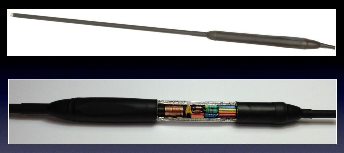
Monopolar Radio-Frequency Antenna with built-in RF conditioning circuitry
